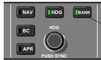
BANK Switch: Used to limit bank angle.
