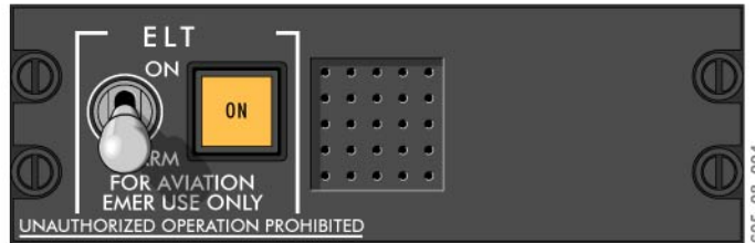
ELT System – Control Panel Figure 08-10-5
