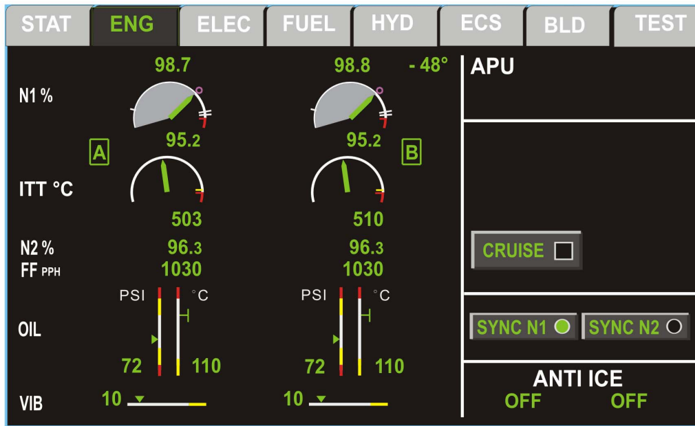
FIGURE 02-70-15-08 MDU ENGINE SYNOPTIC
