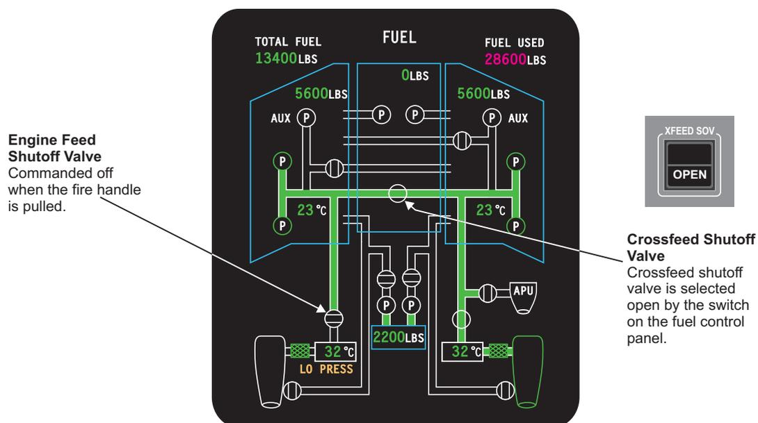
A secondary use of the crossfeed system (as a back-up to the wing transfer system) is to provide means of correcting lateral C of G imbalances, by temporarily inhibiting the flow of fuel from the light side of the airplane. Fuel will then be supplied to both engines from the “heavy” side until lateral fuel balance is within desired limits.
