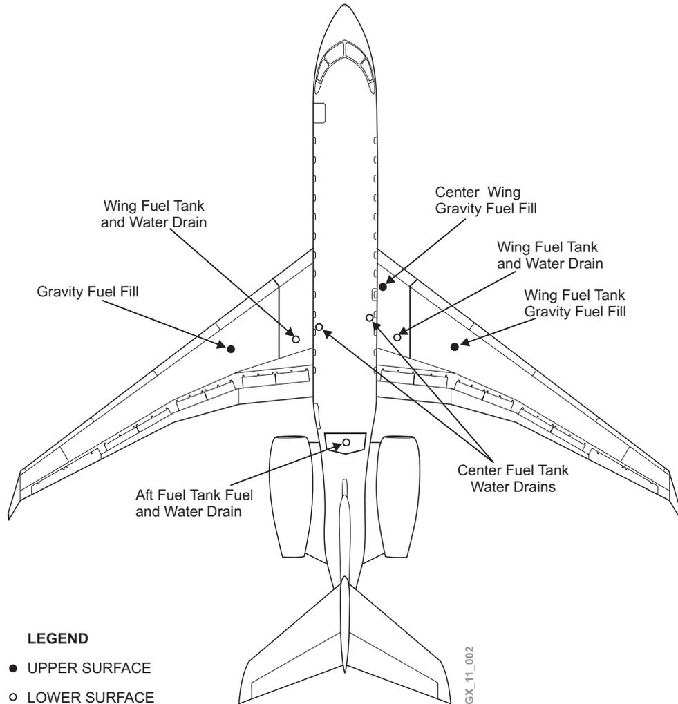
All tanks have flush self-closing water drain valves, installed at various low points, to permit draining of any accumulated water or residual fuel. They are located at the low point of each wing. Three gravity fill caps are provided for wing and center tank gravity refueling.
