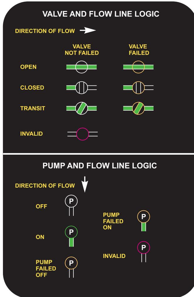
**FUEL SHUTOFF VALVE DISPLAYS**
