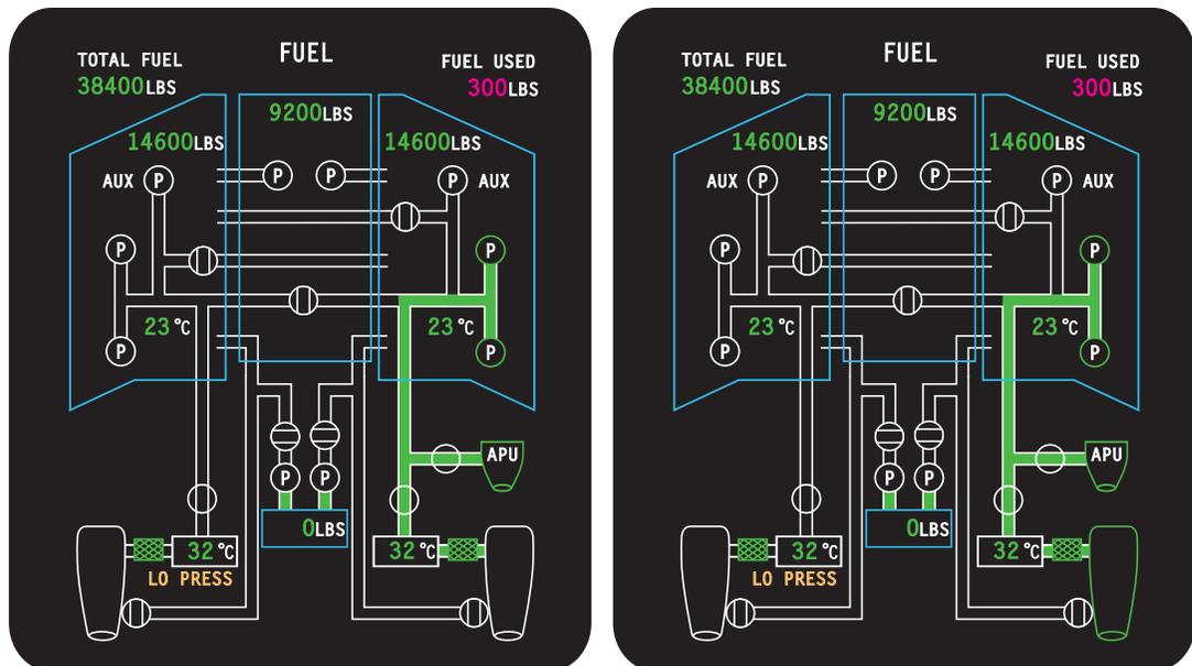
The FUEL synoptic page below represents airplane configuration with the APU shut down, both engines on, the AC pumps running, and the DC pumps on standby.
