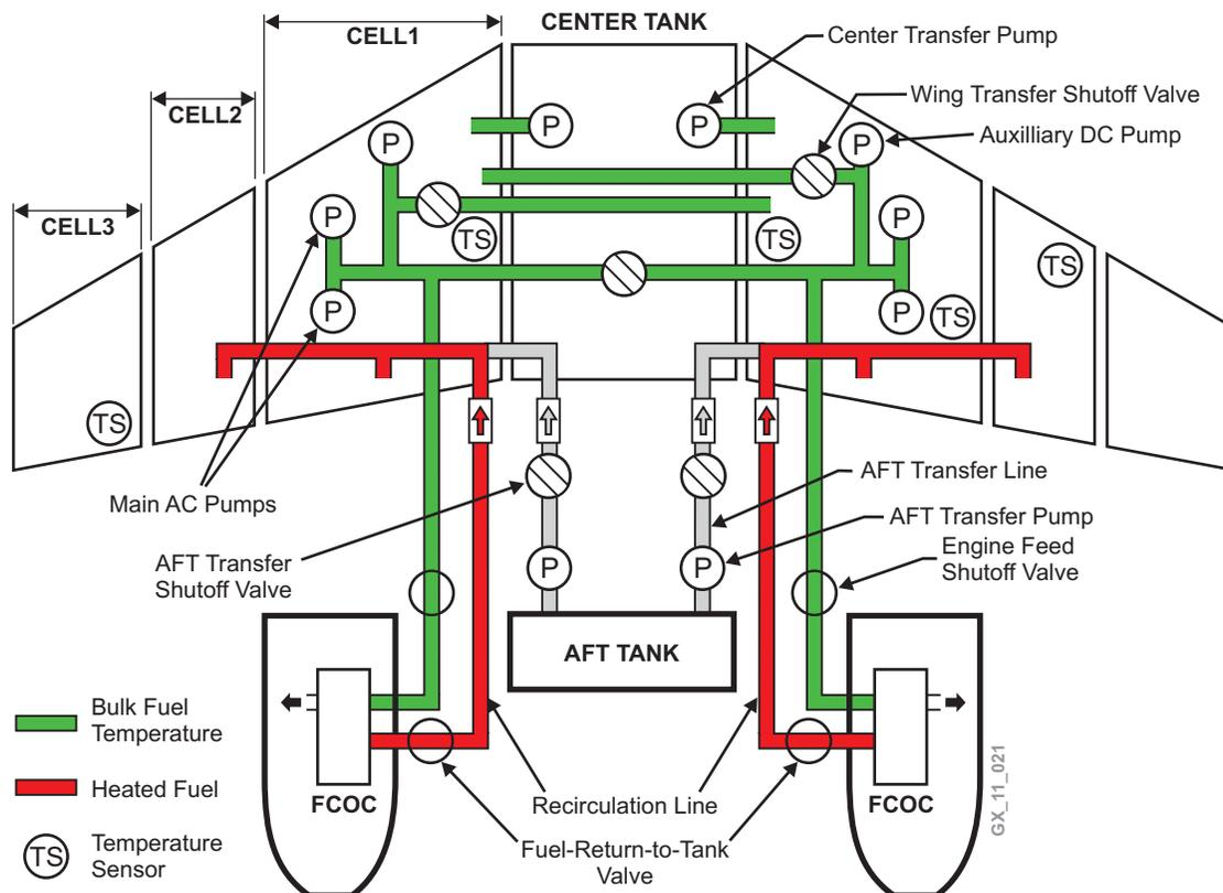
The wing fuel tanks are fitted with many fuel temperature sensors; the left wing has two and the right wing has three. With the Fuel Management and Quantity Gauging Computer (FMQGC) reads all temperature sensors but will display only the lowest temperature. When the Fuel Recirculation system is ON, the FMQGC computer reads the inboard temperature sensor as it will be the one who reads the highest temperature.
