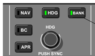
BANK Switch: Used to limit bank angle.
