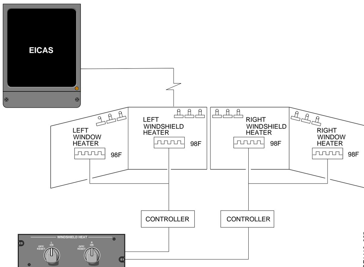
The windshield construction is laminated, stretched acrylic mainplies, which incorporate a gold conductive film as the de-icing heater element. The windshield also includes three temperature sensor elements, one for controlling and monitoring and two spares.
