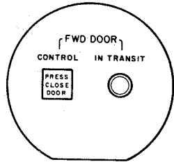
EXTERIOR FWD DOOR CONTROL PANEL
