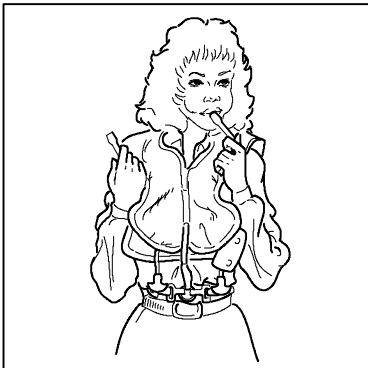
7. Should it become necessary, life vest can be orally inflated by blowing into red oral inflation tubes.
