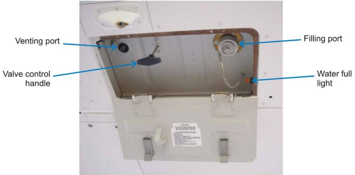
FIGURE 02-38-15-05 SERVICE PANEL DOOR
