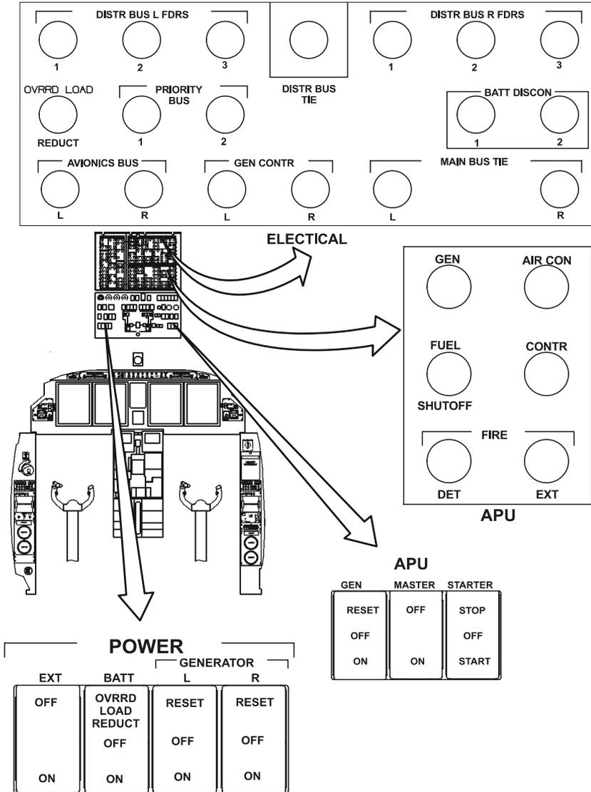
Figure 7-24-3. Electrical System Controls
