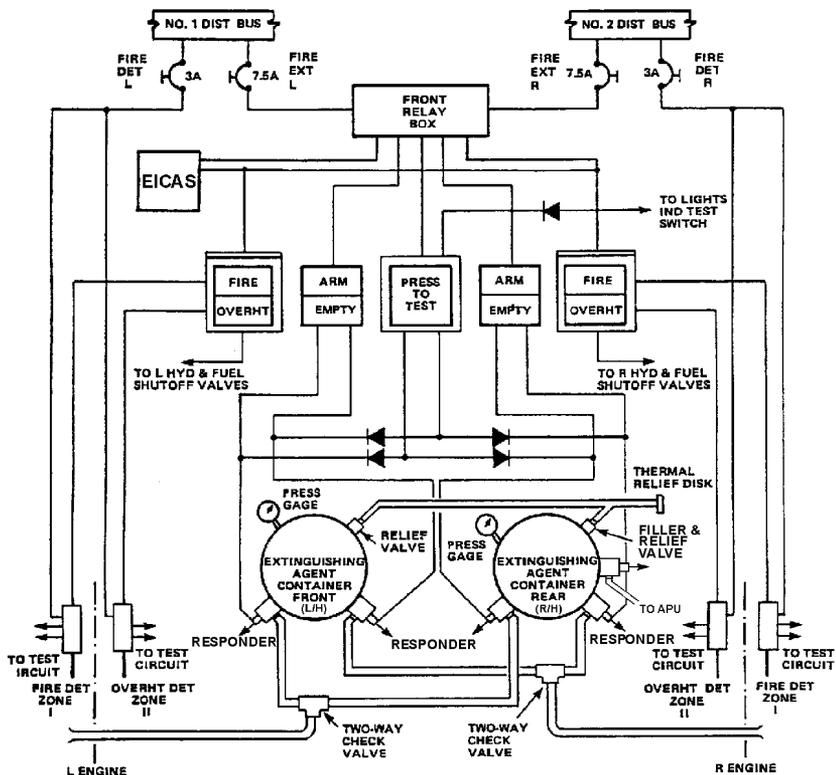
Figure 7-26-1. Engine Fire Protection System - Schematic
