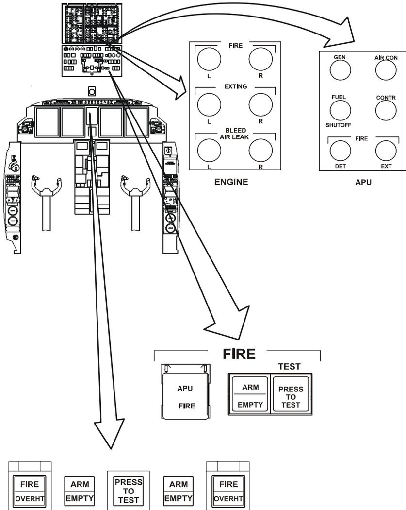
Figure 7-26-3. Fire Protection System Controls and Indicators
