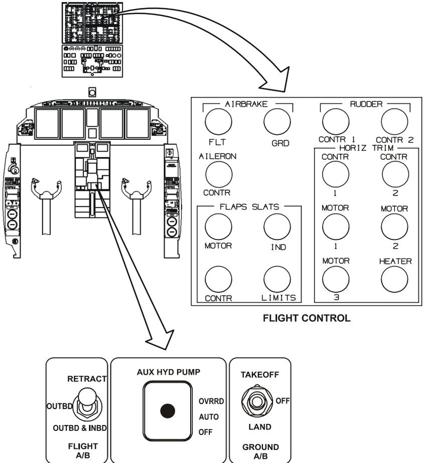
Figure 7-27-5. Air Brakes Controls
