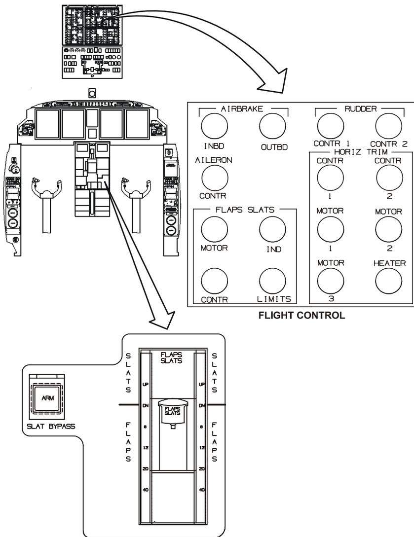
Figure 7-27-4. Flaps / Slats Controls
