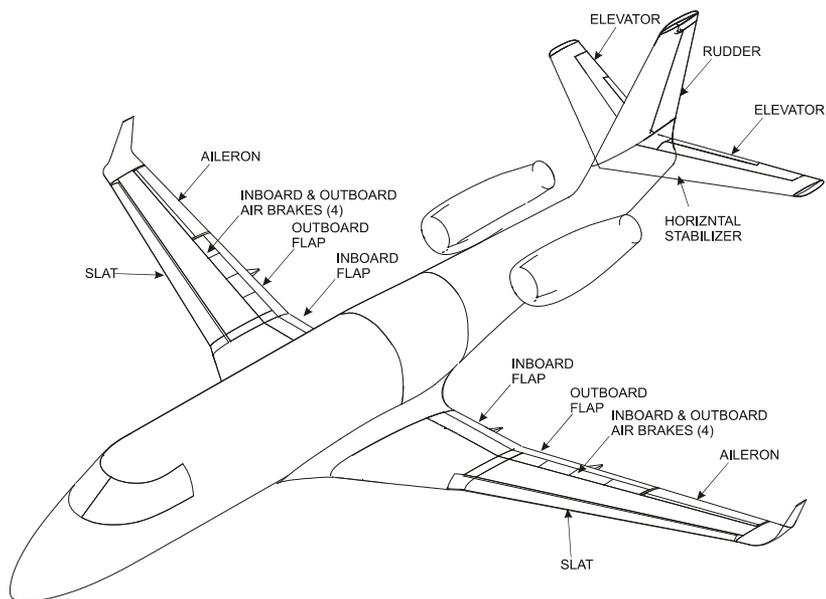
Figure 7-27-1. Flight Controls
