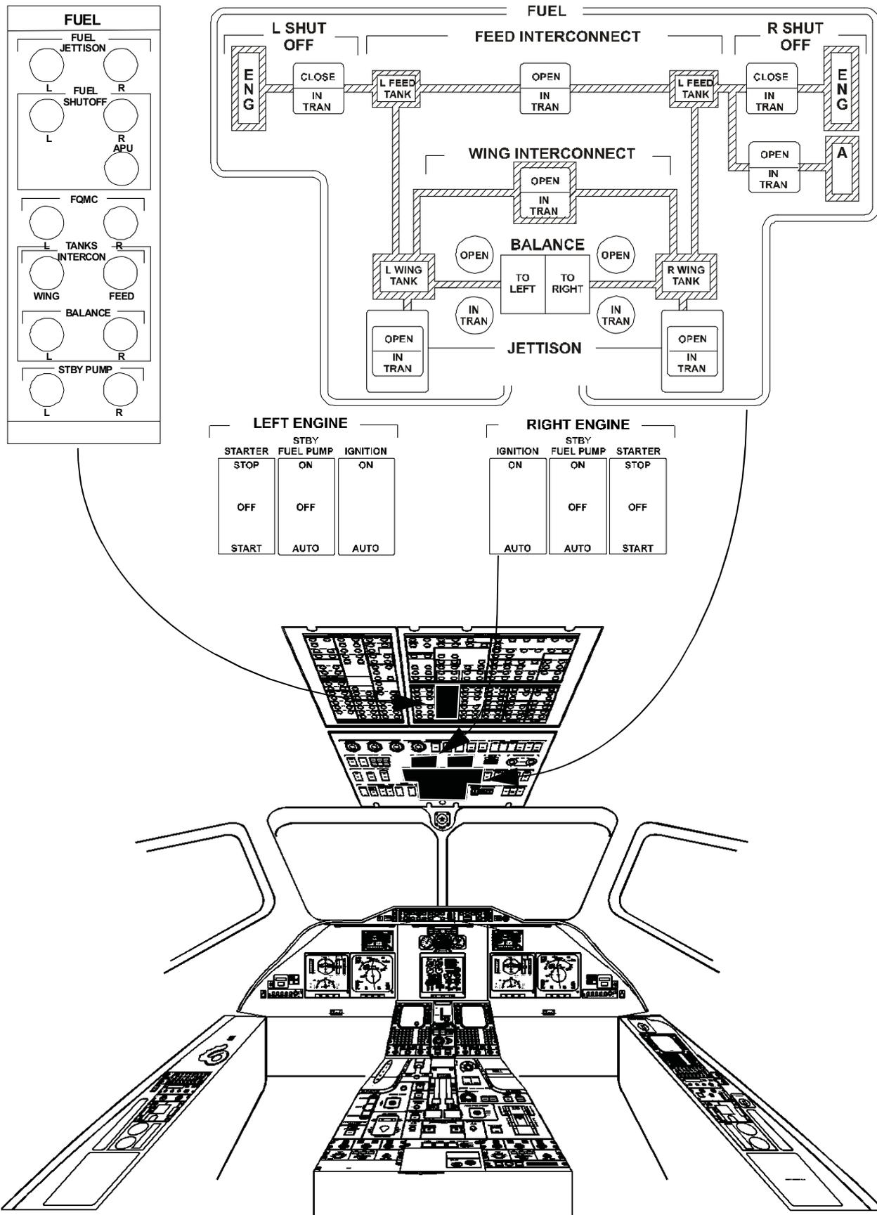
**Figure 5-9. Fuel System Controls and Indicators**
