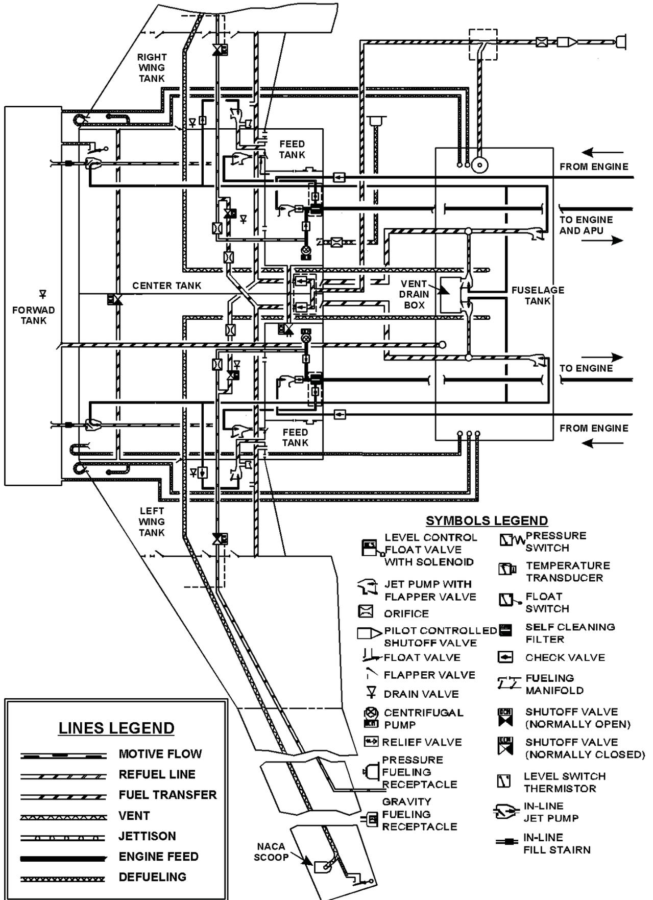
**Figure 5-4. Fuel System - Schematic (Sheet 1 of 2)**
