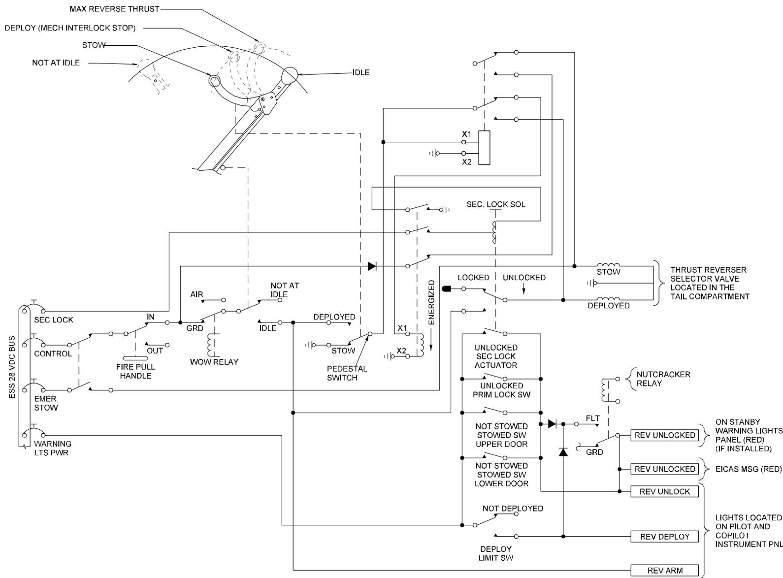
Thrust Reverser Simplified Schematic (Airplanes Having ASC 18, Airplanes SN 1000 - 1143 Excluding SN 1034 Having ASC 166 / 166A and Airplanes SN 1034, 1144 and Subsequent)
