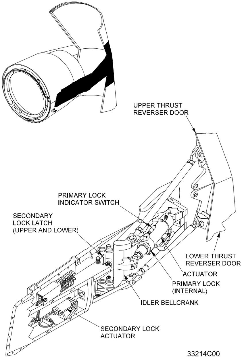
Thrust Reverser Components
