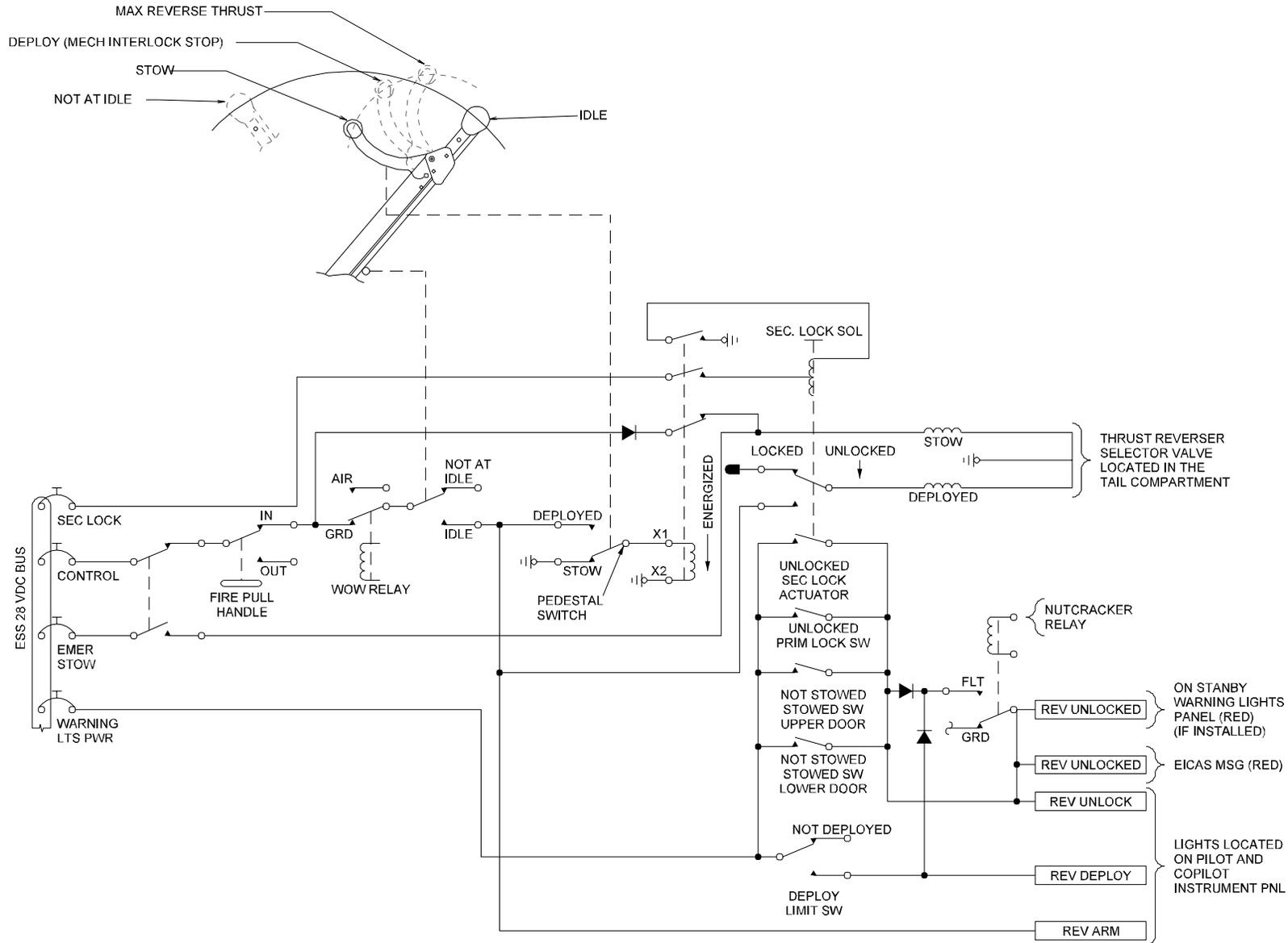
Thrust Reverser Simplified Schematic (Airplanes SN 1000 - 1143 Excluding SN 1034 Not Having ASC 166 / 166A)
