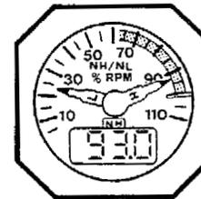
**HIGH-PRESSURE SPOOL SPEED/LOW PRESSURE SPOOL SPEED INDICATOR (N<sub>H</sub>/N<sub>L</sub>)**
