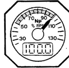
**PROPELLER SPEED INDICATOR (N<sub>p</sub>)**
