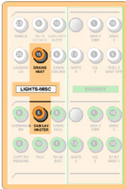
FIGURE 02-38-20-00 OVERHEAD PANEL CIRCUIT BREAKERS
